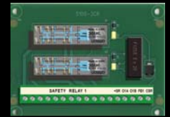
5100-3C Safety Relay Module
