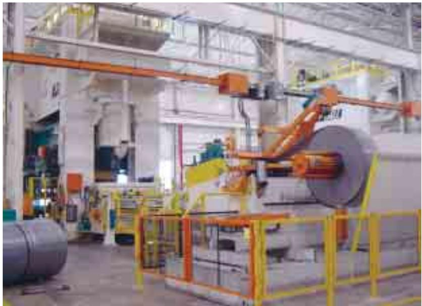
**Beginning a servo-feed setup, proper alignment starts with the die, which should be squared to the centerline of the bolster. Next, the feedline must sit square to, and be centered on, the bolster centerline.**
