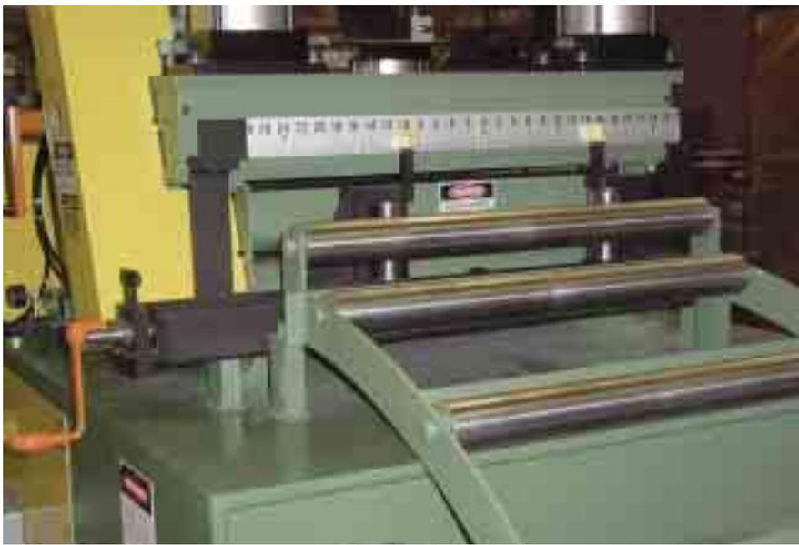
**This feed has a special scale. The vertical guides have pointers that the operator aligns on each side to the material width. This scale aids in aligning the material square to the die and on the centerline of the press bolster.**
