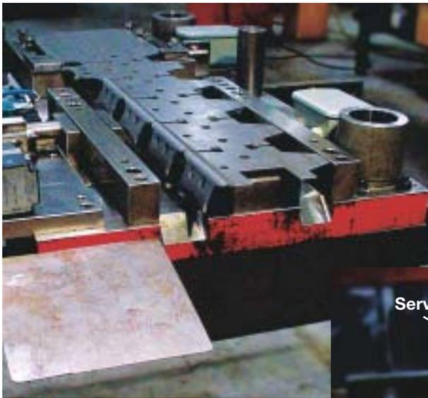
This Ultra Tool and Manufacturing progressive die (below) incorporates an analog sensor (at station six) to measure inside bend angle and a servomotor (station five) to adjust the form if required to bring the part back to nominal. The air cylinder controls the bad-part diverter to avoid shipping defective parts to the customer. The photo to the left shows the die with the strip in place.
