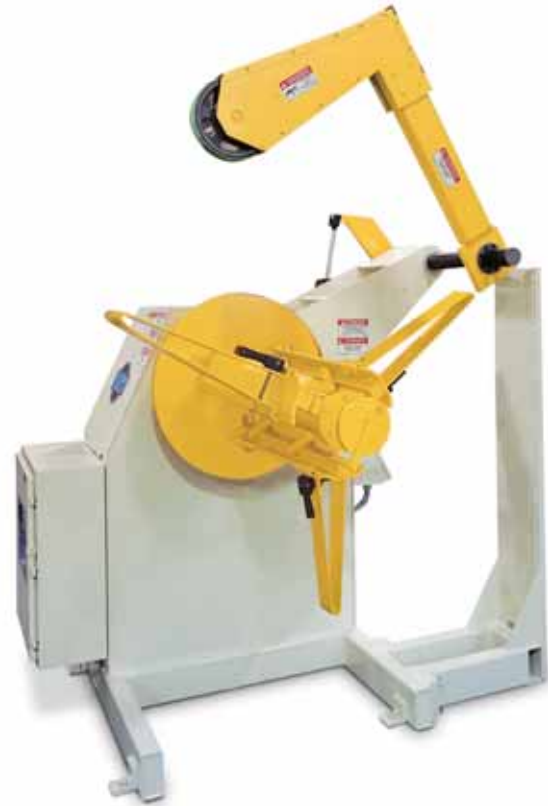
■ Standard 6,000# Series reel configured for "pull-off" application with manual hand crank expansion, optional air operated coil hold down arm with motorized end wheel, and coil clockspring guard.
