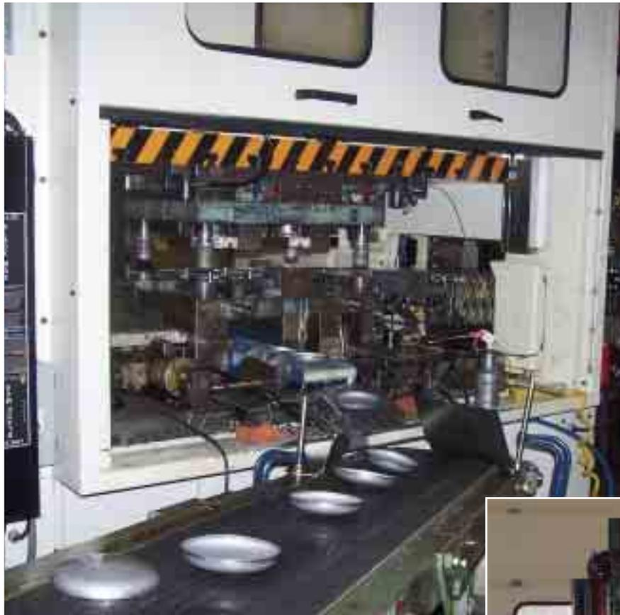
Presence-sensing light curtains on these mechanical presses establish the primary point-of-operation guarding. When establishing the distance at which to establish the light curtain from the press, stampers should use a formula that accounts for the penetration factor, which considers the minimum size of an object that a presence-sensing device can still detect 100 percent of the time anywhere in the sensing field.
