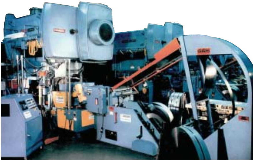
Cradle feed lines minimize cost and use less floor space than conventional lines, but are less flexible.
