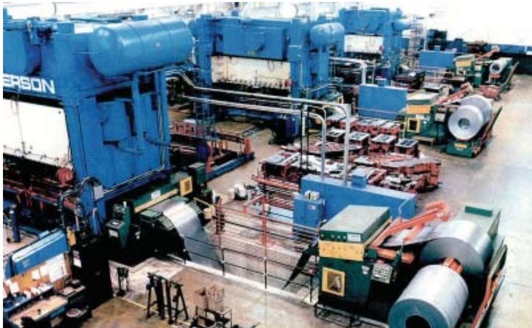
While offering the most flexible arrangement, this conventional feed line also carries the highest cost and uses the most floor space.
