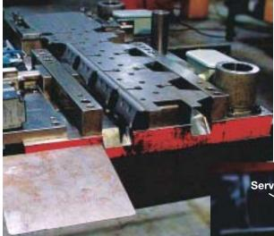
This Ultra Tool and Manufacturing progressive die (below) incorporates an analog sensor (at station six) to measure inside bend angle and a servomotor (station five) to adjust the form if required to bring the part back to nominal. The air cylinder controls the bad-part diverter to avoid shipping defective parts to the customer. The photo to the left shows the die with the strip in place.
