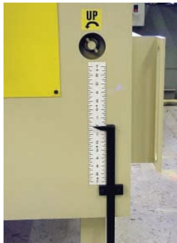
Adjusting passline height takes more time than necessary when the company fails to provide a scale or reference to assist in setup, requiring the operator to eyeball the die and feed, a cumbersome process dependant upon operator skill. Use of a reference scale—an easy-to-read scale and pointer—allows the operator to quickly return the feed to a predetermined height.
