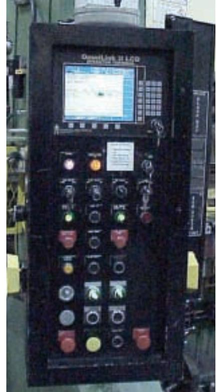
To make the press operator's job easier and eliminate wasted steps during setup, TCR Integrated Stamping Systems expanded a press control to integrate control of ancillary equipment such as the straightener and feeder. Photo courtesy of Link Systems.
