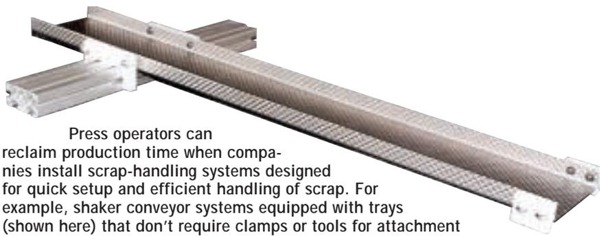
Press operators can reclaim production time when companies install scrap-handling systems designed for quick setup and efficient handling of scrap. For example, shaker conveyor systems equipped with trays (shown here) that don't require clamps or tools for attachment can minimize setup time. Photo courtesy of Dura-Glider.
